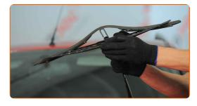
Remove the blade from the wiper arm.
