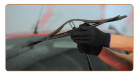
Remove the blade from the wiper arm.
