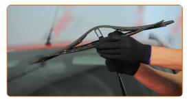
Remove the blade from the wiper arm.
