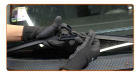
Remove the blade from the wiper arm.
