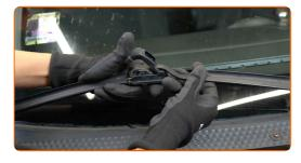
Remove the blade from the wiper arm.
