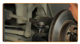
Tighten the fastening nut connecting the tie rod end to the steering knuckle. Use a drive socket #15. Use a torque wrench. Tighten it to 40 nm torque.
