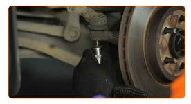
Clean the lock nut that connects the tie rod to the tie rod end. Use a wire brush. Use WD-40 spray.
