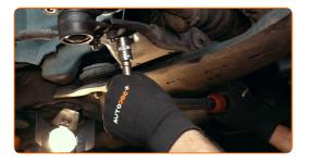
Tighten the lower fastening of the shock absorber. Use a drive socket #15. Use a torque wrench. Tighten it to 83 Nm torque.
