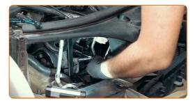
Connect the coolant hoses to the thermostat housing.
