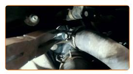
Screw on the fastener of the power steering pipe bracket.
