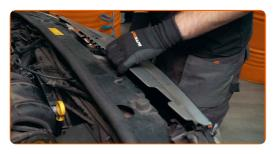
36 Screw in the fastener of the radiator grille.
