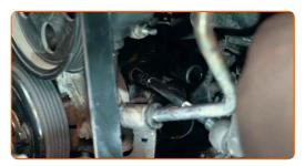
Remove the thermostat housing together with the thermostat.
