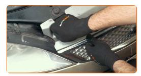
Remove the coolant reservoir cap.
