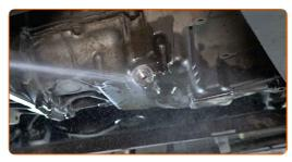
Screw in the new drainage plug and tighten it. Use a drive socket #21. Use a torque wrench. Tighten it to 26 nm torque.
