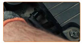
Remove the air intake pipe.
