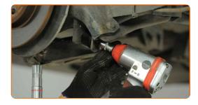
Tighten the top shock absorber fastening. Use a combination spanner #18. Use a drive socket #15. Use a torque wrench. Tighten it to 84 Nm torque.
