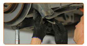
Tighten the lower fastener of the shock absorber. Use a drive socket #18. Use a torque wrench. Tighten it to 120 Nm torque.
