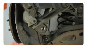
Unscrew the upper fastener of the shock absorber. Use a combination spanner #18. Use a drive socket #15. Use a ratchet wrench. Use a tap wrench.
