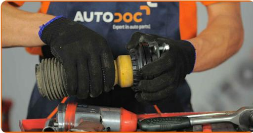
**43** Tighten the shock strut piston rod nut. Use a combination spanner #18. Use HEX No.H6. Use a torque wrench. Tighten it to 58 Nm torque.
