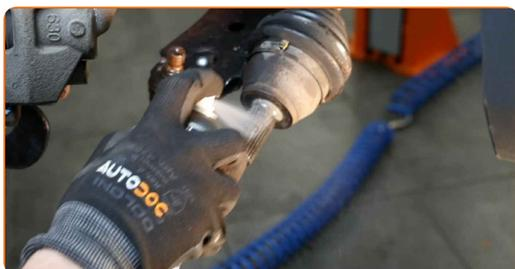
**54** Mount the drive shaft into the wheel hub.
