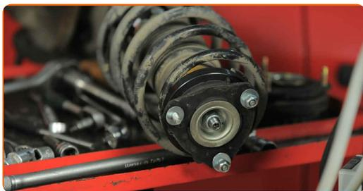
**46** Install the shock strut into the wheel arch.
