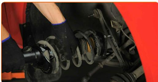
**47** Screw the top fastening of the shock strut mount.
