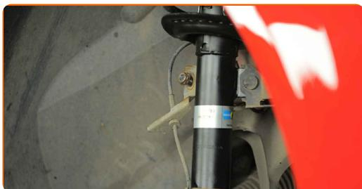
**70** Tighten the fastener connecting the stabilizer link to the shock strut. Use a combination spanner #17. Use HEX No.H5. Use a torque wrench. Tighten it to 48 Nm torque.
