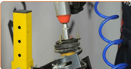
**41** Remove the shock absorber mount, boot and bump stop. Use a flat screwdriver.
