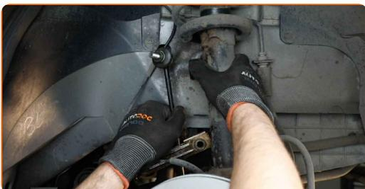
**12** Clean the fastener of the driveshaft. Use a wire brush. Use WD-40 spray.
