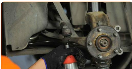
**23** Disconnect the tie rod end from the steering knuckle. Use a ball joint puller.
