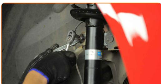
**71** Attach the ABS sensor connector.
