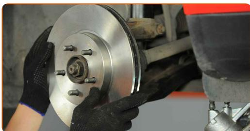
**60** Clean the mounting seats of the caliper and its bracket. Use a wire brush. Use WD-40 spray.
