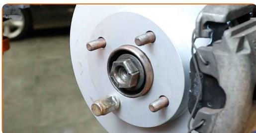
**73** Tighten the drive shaft nut. Use a drive socket #32. Use a torque wrench. Tighten it to 290 Nm torque.
