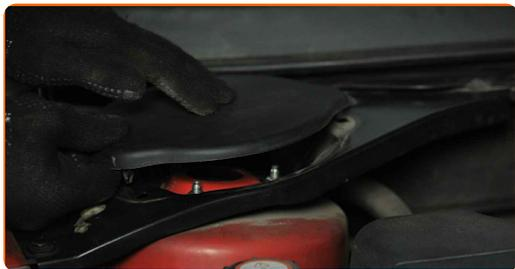
**50** Remove the fender protection cover.
