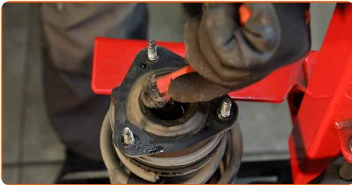
**40** Remove the strut piston rod nut. Use a combination spanner #18. Use HEX No.H6. Use a ratchet wrench.
