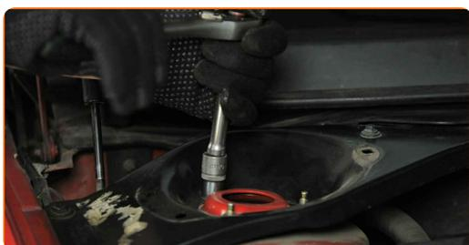
**49** Install the protective shock absorber mounting cap.
