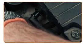
Remove the air intake pipe.
