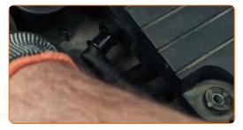
Remove the air intake pipe.
