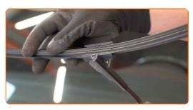
Remove the blade from the wiper arm.
