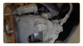
19 Install the brake caliper retaining spring.
