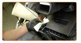
Replacement: engine oil and filter – FORD Kuga Mk1 (C394). AUTODOC recommends:
