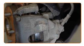
19 Install the brake caliper retaining spring.
