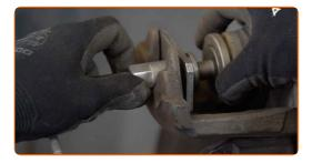
Check the brake caliper bracket, brake caliper guide pins and boots. Clean them. Replace, if necessary. Use a wire brush. Use a brake cleaner.
