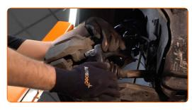
Remove the brake caliper.
