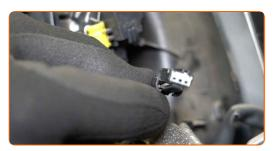
Detach the mirror adjuster connector from the door.
