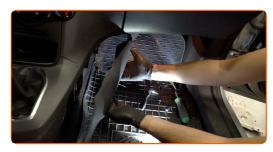
Reinstall the clips of the plastic side panel.
