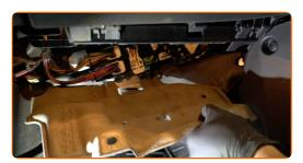
Remove the clips from the plastic side panel. Use a clip removal tool.
