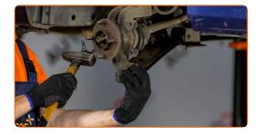
Clean the fasteners connecting the shock strut to the steering knuckle. Use a wire brush. Use WD-40 spray.
