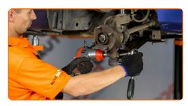
38 Install the brake disc.
