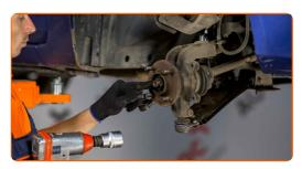
Unscrew the wheel hub axle nut. Use a drive socket #32.
