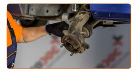
Press the wheel hub out from the tapered roller bearing. Use a bush and bearing driver set. Use a hammer.
