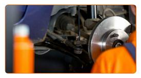
Tighten the fastening nut connecting the tie rod end to the steering knuckle. Use a drive socket #17. Use a torque wrench. Tighten it to 48 nm torque.
