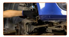
Disconnect the lower arm from the steering knuckle. Use a crowbar.
