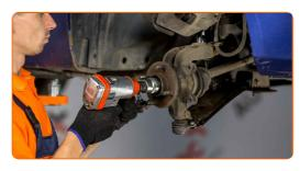
Remove the drive shaft. Use a hammer.
