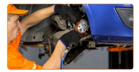
Tighten the hub. Use a drive socket #32. Use a torque wrench. Tighten it to 290 nm torque.
