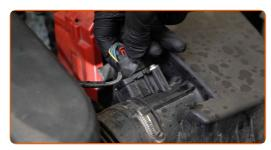
Detach the air intake hose clamp. Use a drive socket #7. Use a ratchet wrench.
