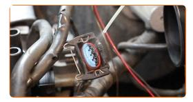
Plug in the ignition coil connector.
