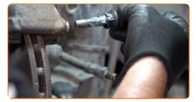
Tighten the brake caliper fasteners. Use HEX No.H7. Use a torque wrench. Tighten it to 35 Nm torque.
