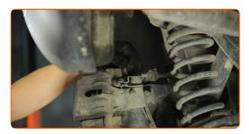
Install the brake caliper retaining spring. Use a flat screwdriver.
