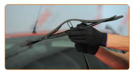
Remove the blade from the wiper arm.
