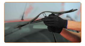
Remove the blade from the wiper arm.
