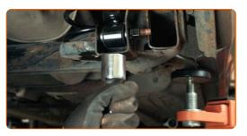
Tighten the lower fastener of the shock absorber. Use a drive socket #15. Use a torque wrench. Tighten it to 115 Nm torque.
