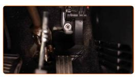
Remove the clips from the plastic side panel. Use a clip removal tool.
