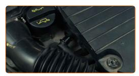
Remove the air filter housing.
