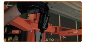
Connect the fuel supply lines to the fuel filter.
