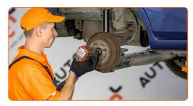
10 Remove the brake drum.
