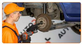
9 Unscrew the hub bearing mounting. Use a drive socket #30.
