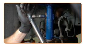
71 Fasten the brake hose on the strut.
