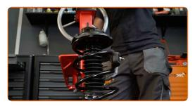
Treat the shock strut rod. Use copper grease.
