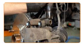
Unscrew the upper fasteners of the shock strut (3 pieces).
