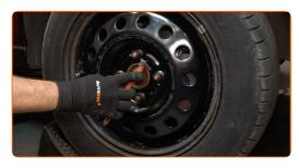
Loosen the fastener of the driveshaft. Use a drive socket #32. Use a tap wrench.
