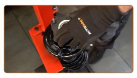
Tighten the shock strut piston rod nut. Use a drive socket #19. Use HEX No.H7. Use a torque wrench. Tighten it to 55 Nm torque.
