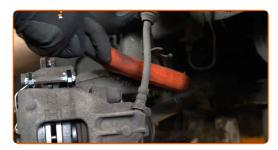
Unscrew the lower fastener connecting the shock strut to the steering knuckle. Use a drive socket #15. Use a ratchet wrench. Use a tap wrench.
