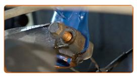
Screw in the fastener that connects the shock strut to the steering knuckle. Use a drive socket #15. Use a ratchet wrench.
