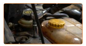
6 Clean the fastener of the driveshaft. Use a wire brush. Use WD-40 spray.
