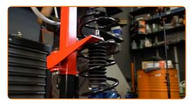
Install the upper strut mount and the strut mount bearing.
