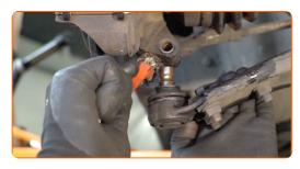
Connect the ball joint to the steering knuckle.
