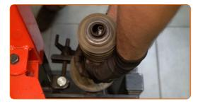
Install the boot and a bump stop onto the shock absorber.
