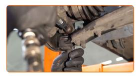
Tighten the ball joint fastener. Use a drive socket #15. Use a torque wrench. Tighten it to 47 Nm torque.
