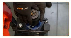
Install the spring on the shock absorber.
