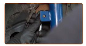
Tighten the stabiliser link fastener. Use a combination spanner #15. Use a drive socket #15. Use a ratchet wrench.
