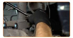
Unscrew the fastener connecting the drive shaft to the wheel hub.
