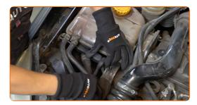
Release the coolant reservoir retainers. Use a flat screwdriver.
