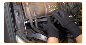
Remove the support from under the engine.
