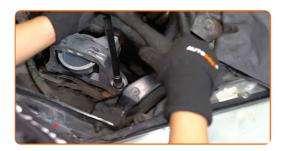
Screw in the upper fastener of the engine mount. Use a drive socket #16. Use a ratchet wrench.
