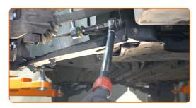
Tighten the fastener connecting the stabilizer link to the shock strut. Use a drive socket #15. Use a torque wrench. Tighten it to 50 Nm torque.
