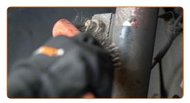
Unscrew the fastener connecting the stabilizer link to the stabilizer bar. Use a combination spanner #17. Use a drive socket #17. Use a ratchet wrench.
