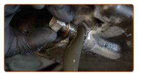
Replacement: engine oil and filter – FORD Focus Mk4 Turnier (HP). AUTODOC recommends:
