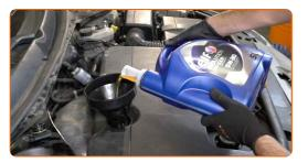
Replacement: engine oil and filter – FORD Focus Mk4 Hatchback (HN). Tip from AUTODOC:
