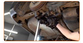
Tighten the shock absorber mount fasteners. Use a drive socket #10. Use a torque wrench. Tighten it to 25 Nm 24 torque.
