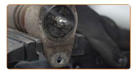
Remove the shock absorber piston rod fastening. Use a combination spanner #13. 14
