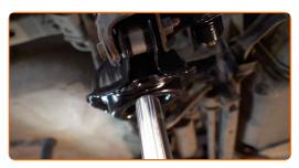
Clean the wheel rim mounting seat. Use a wire brush. Treat the contacting surface. Use copper grease.
