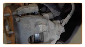
Install the brake caliper retaining spring.
