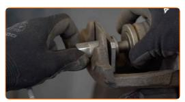
Check the brake caliper bracket, brake caliper guide pins and boots. Clean them. Replace, if necessary. Use a wire brush. Use a brake cleaner.
