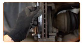
Replacement: brake pads – FORD Focus Mk3 Box Body / Hatchback. Professionals recommend:
