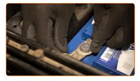
Screw in the positive battery terminal fastener. Use a 10 mm socket. Use a ratchet wrench.
