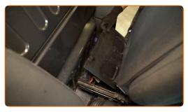
Unscrew the negative battery terminal fastener. Use a 10 mm socket. Use a ratchet wrench.
