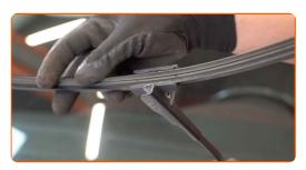
Remove the blade from the wiper arm.
