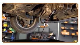
Replacement: engine oil and filter – FORD Focus Mk2 Hatchback (DA\_, HCP, DP). Tip:
