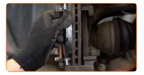
Replacement: brake pads – FORD Focus Mk2 Hatchback (DA\_, HCP, DP).
