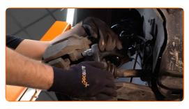
Remove the brake caliper.
