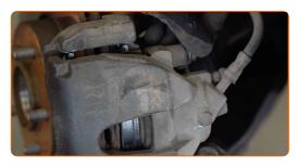
Install the brake caliper retaining spring.
