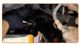
Connect the ball joint to the steering knuckle.
