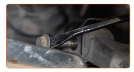
Unscrew the rear arm fastener. Use a drive socket #15. Use a ratchet wrench.
