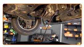
Replacement: engine oil and filter – FORD Focus Mk2 Estate (DA\_, FFS, DS). Tip:
