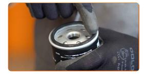
Screw the new filter into its place. Use the 76-30F socket. Use a torque wrench. Tighten it to 18 nm torque.
