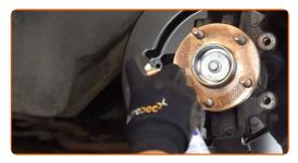
13 Install the brake disc.
