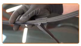
Remove the blade from the wiper arm.
