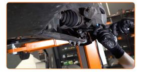
Unscrew the fastening nut, remove the control arm from the steering knuckle, using a ball joint puller.
