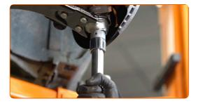
20 Install the fastening nut of the ball joint.
