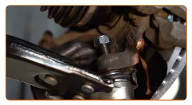
21 Install the rear fastener of the arm.
