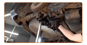
24 Tighten the shock absorber mount fasteners. Use a drive socket #10. Use a torque wrench. Tighten it to 25 Nm torque.
