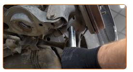
Tighten the lower fastener of the shock absorber. Use a drive socket #16. Use a torque wrench. Tighten it to 103 Nm torque.
